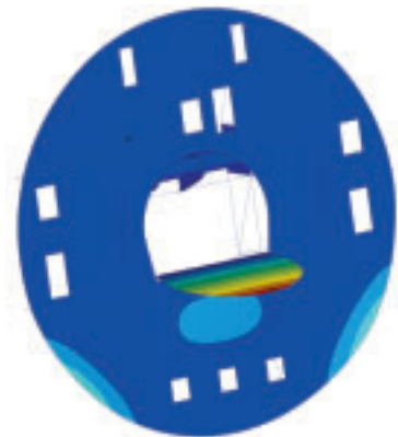
The eye structure is a composite, a steel frame with a wood outer surface. Using the nonlinear capabilities of software from ANSYS, ZT Lener was able to accurately predict the physics involved in this complex analysis.
