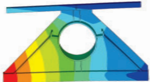
The triangular brackets that connect the eye to the rotating shaft are critical parts of the steel support structure. Based on the analysis results of the triangular support, engineers changed the wall thicknesses and positions of the stiffeners on the brackets in order to reduce deformations and stresses to safe levels.
