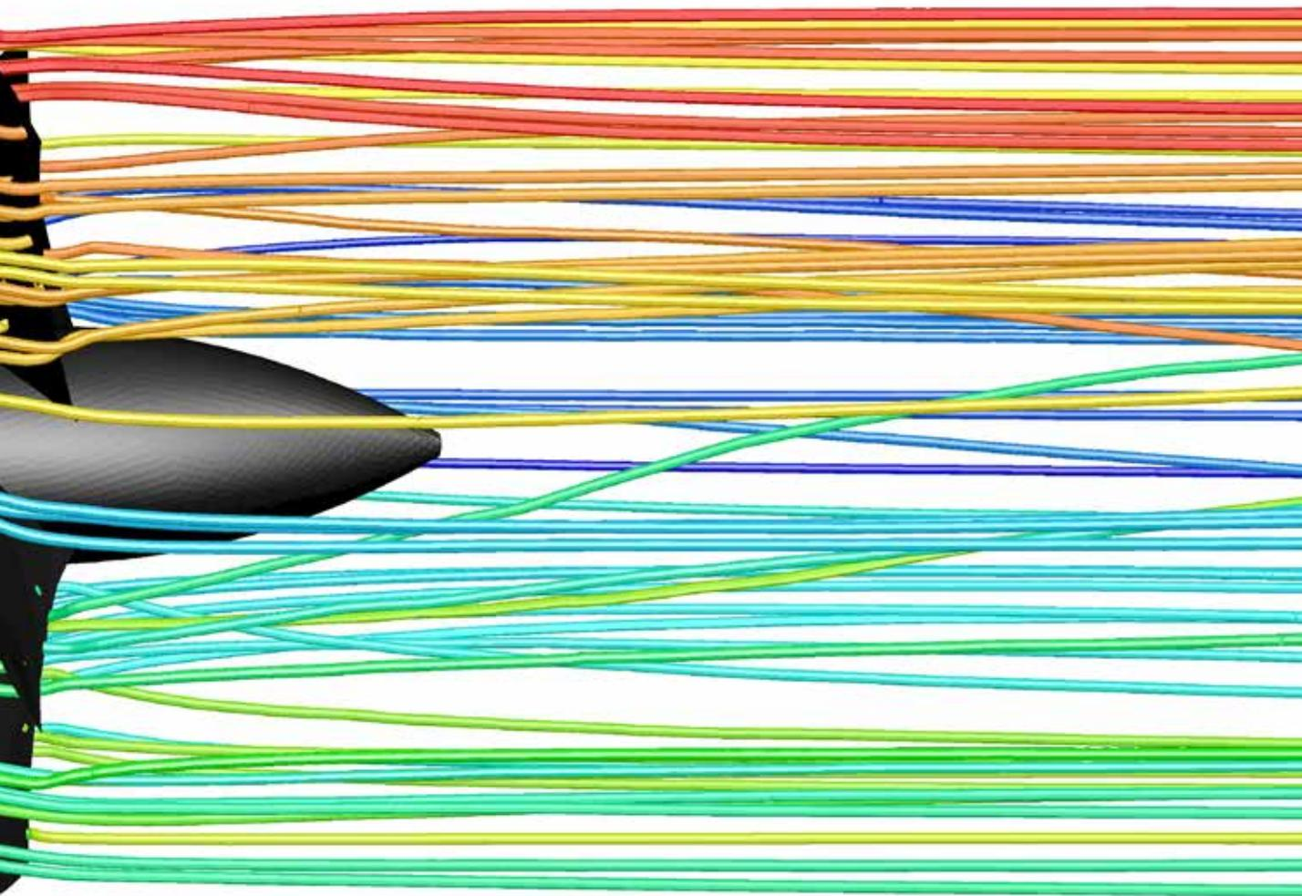
▲ Flow streamlines generated by both rotors show how tangential flow is canceled out.
