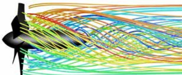
▲ Flow streamlines generated by upstream rotor in isolation show high tangential flow.
