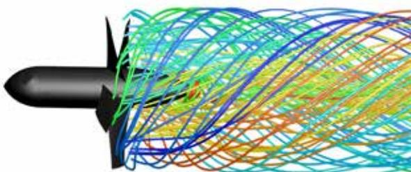
▲ Flow streamlines generated by downstream rotor in isolation show high tangential flow.
