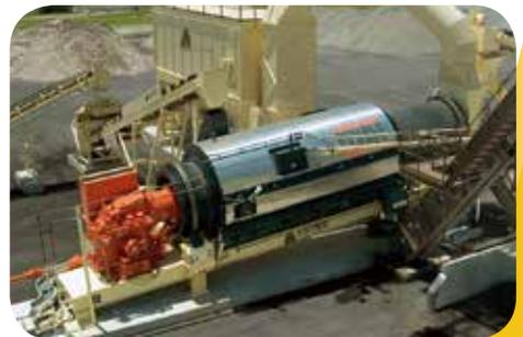
**A**stec Industries continually works to improve the efficiency of aggregate dryers for asphalt production to reduce energy consumption and save energy costs for customers in this growing industry. Direct observation of the dryer drum in operation is difficult, so simulation offers the best opportunity to experiment with new designs.
