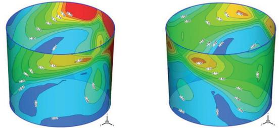
The high level of shear stress on the original ladle (red region on the left) indicates localized regions of high shear stress which lead to very high refractory erosion. Because there is less variation in shear stress in the improved ladle (right), the lining life could be significantly increased.
