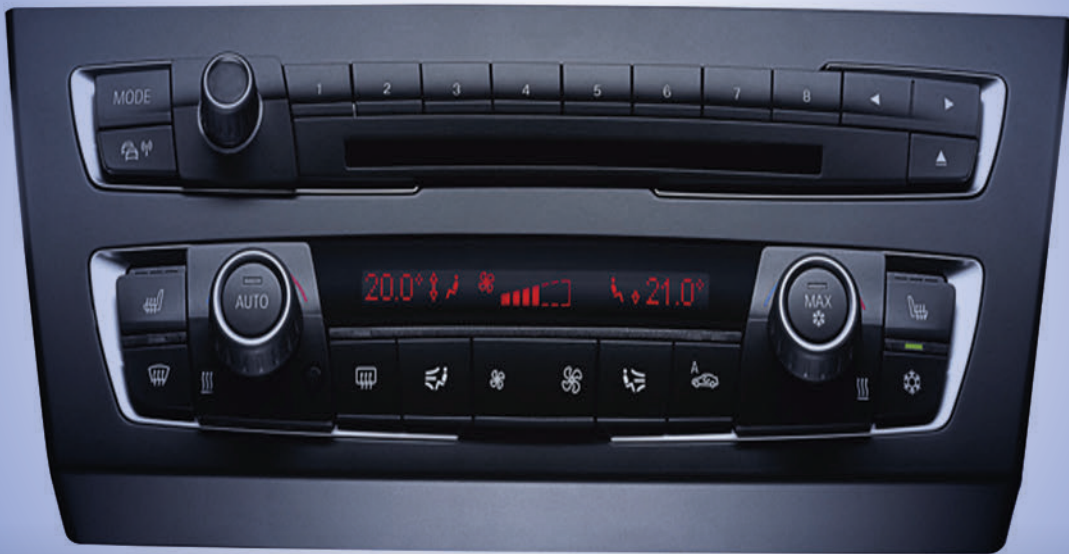
Audio system that uses snap-fit assembly
