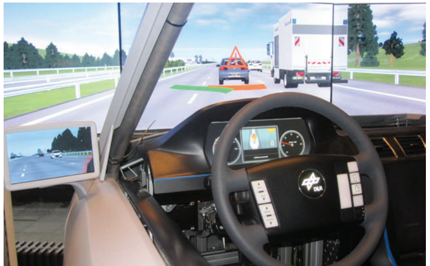
▲ HMI on heads-up display for highly automated driving
