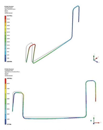
Total deformation (top) and maximum combined stress (bottom) at true scale
