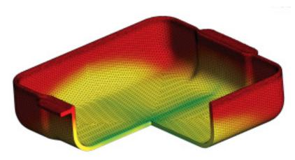
Temperature distribution during the cooling of a dish. Using the Narayanaswamy model, it is possible to detect the peak stress related to the emergence of defects at the core of virtual glass products.
