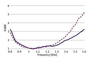
Measurements of final antenna design show that it closely matches performance of conventional antenna at frequencies of interest between 1 and 1.2 GHz.
