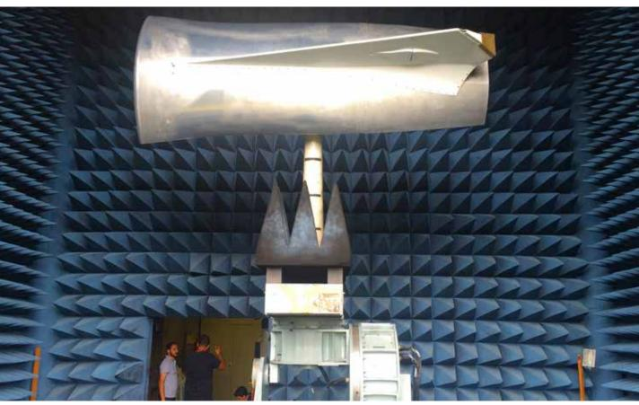
Prototype of aircraft dorsal fin tested in anechoic chamber
