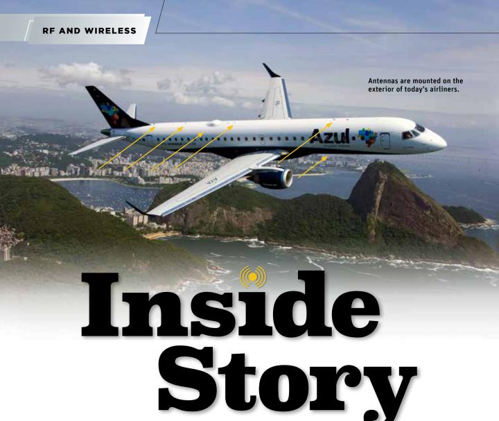
The scores of antennas extending from the surface of today's jet airliners create drag that adds to fuel consumption. Brazilian National Institute of Telecommunications (Inatel) and Embraer engineers have been developing new ways of installing antennas that could save fuel. With ANSYS simulations, engineers can predict the performance of proposed installations without the time and expense of building prototypes.
