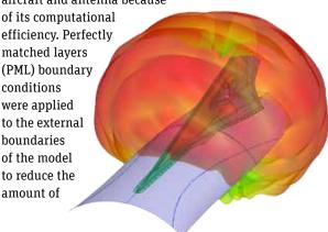
ANSYS HFSS simulation results show radiation amplitude field generated by antenna designed within fuselage.
