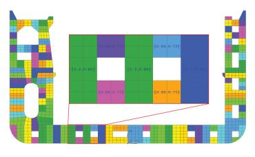
The results can be presented over sections (frames/longitudinals/decks) and results which are above the limit are highlighted with red:
