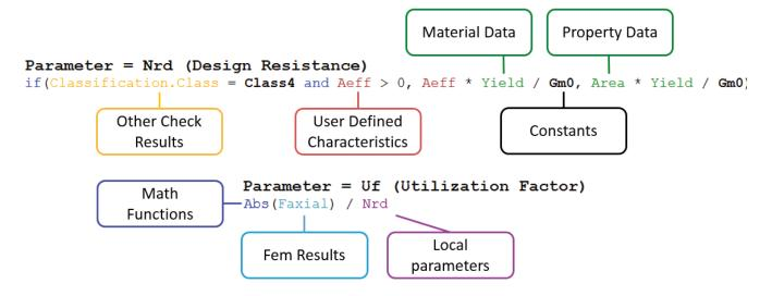
The following example demonstrates a verification of bolted connections. The Axial Force of bolts is compared with the bolt design resistance:
