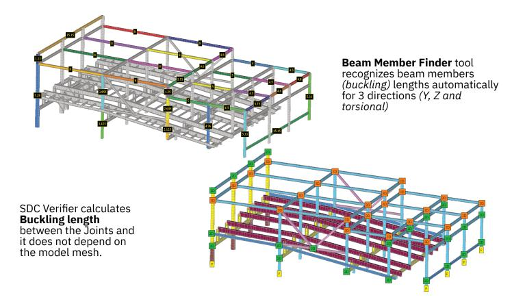
The deflection of members is one of the checks that should be performed for serviceability limit state design. With the help of **Beam Member Finder** tool SDC Verifier automatically recognizes beam member lengths:
