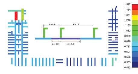
Effective Width — calculates the plate effective width for every load situation. The Effective width is used in the stiffener buckling check according to DNV-RP-C201 2010
