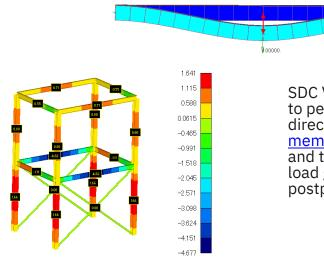
SDC Verifier contains all the necessary tools to perform the deflection check quickly directly within Ansys. The <u>automatic beam</u> <u>member recognition</u>, result transformation and the usage of the envelope results of a load group reduce the calculation and postprocessing time significantly.
