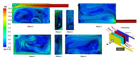
Figure 2. Velocity & Contours on different planes in Z Direction
