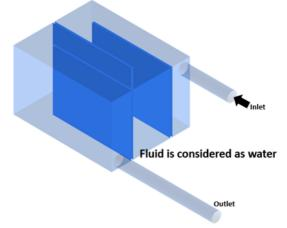
Figure 1. 3D model created in Ansys CAD tool
