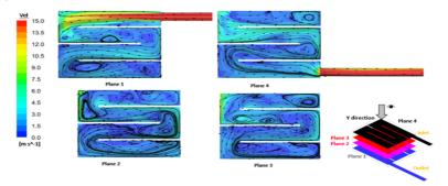
Figure 3. Velocity & Contours on different planes in Y Direction
