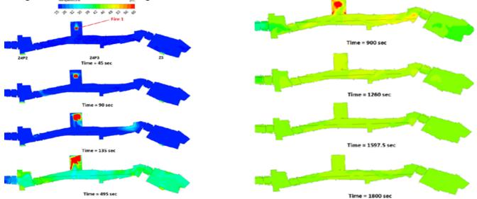
Figure 2 & 3. Shows fire 1 zone, where the fire evolves with time and then decaying gradually. With red being the highest and blue as lowest points of temperature scale.
