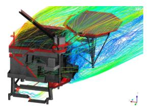
Figure 2. Streamlines of the flow over the helideck
