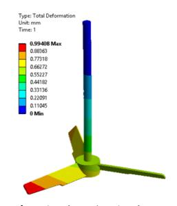
**Figure 2.** Deformation plot of Rotor Blades
