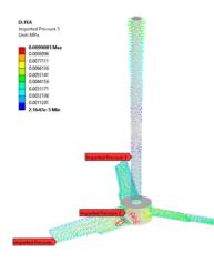
**Figure 1.** Imported Pressure distribution from CFD
