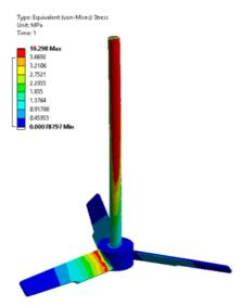
**Figure 3.** Stress contour plot of Rotor Blades
