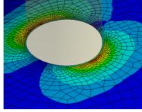
Figure 2. Stress contour plot of global model
