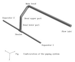
Figure 1. Geometry of the piping system
