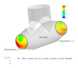
Figure 2. Contour plots representing the flow on each side of the separators
