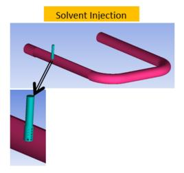
**Figure 2.** The model of piping system and injection pin
