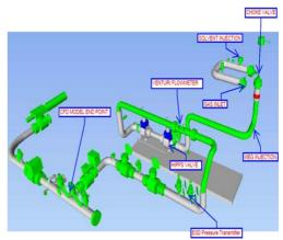
**Figure 1.** Model of injection and gas piping system
