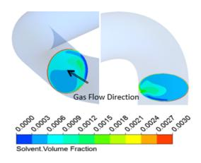
**Figure 3.** Contour plot indicating the Volume fraction in ppm
