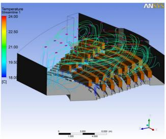
Figure 2. Streamlines colored by temperature
